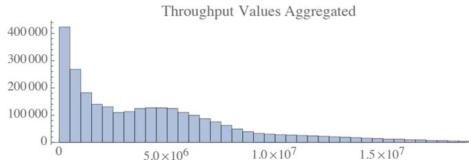
Fig. 2. Histogram of the raw throughput values recorded during all IOzone tests across all system configurations. The distribution is skewed right, with few tests having significantly higher throughput than most others.
